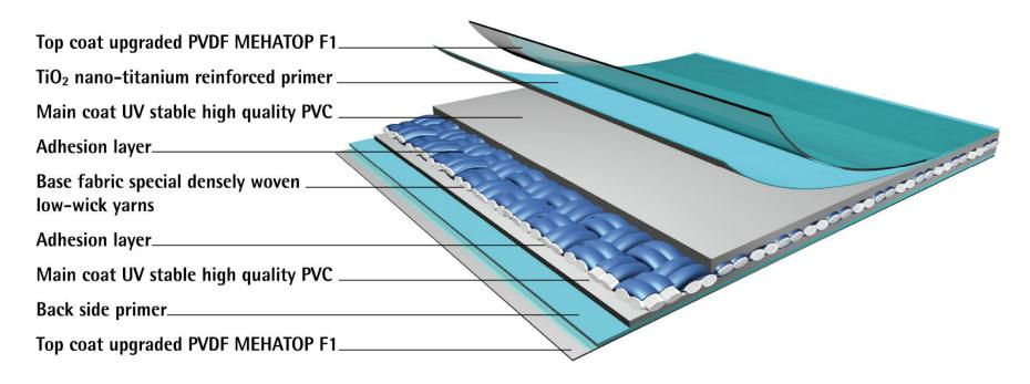
We weave fabrics from high-tenacity polyester yarn before coating it on one of the four state-of-the-art PVC coating lines...
